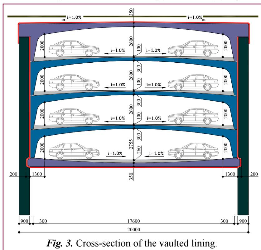
**Fig. 3.** Cross-section of the vaulted lining.
