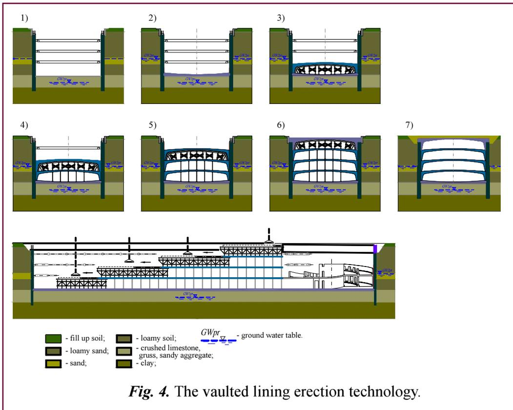
Each of 17.5 m wide sections of this and of subsequently constructed vaults were reinforced with the same type 2.4 m-wide reinforcing space cages.
